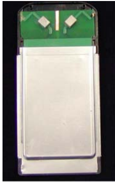
Figure 7. Two-dual band WLAN antennas covering the 802.11a&b bands on a PCMCIA card, UK Patent Application Number 0311361.0
